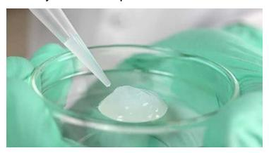
A team of scientists at King Abdullah University of Science and Technology (KAUST), Saudi Arabia has designed electrically conductive hydrogel that takes stretchability, self-healing and strain sensitivity to new limits.
